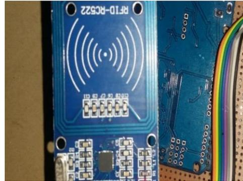
**Fig. 4: RFID MFRC522 reader**
