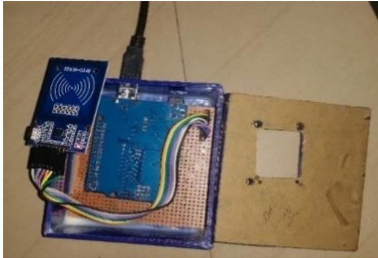
Fig. 8: A serial connection between the RFID Tag and reader.
