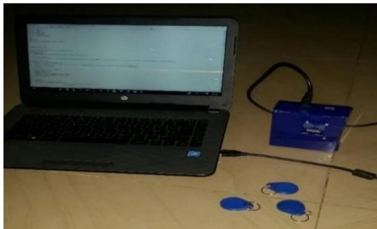
Fig. 9: RFID system connection to the computer through the USB port.
